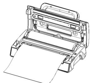
Put one end of the bag on top of the sealing bar, but not enter the vacuum chamber.
