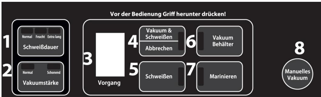
**1 Sealing time (Schweißdauer):** Three buttons for choosing the best bag seal time
