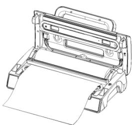
Put down the cutter rack and make sure it is on the right place of the bags, then slide the cutter from one end to the other end to cut the bag.
