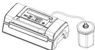
Wipe canister cover, canister base and ensure they are clean and dry.
