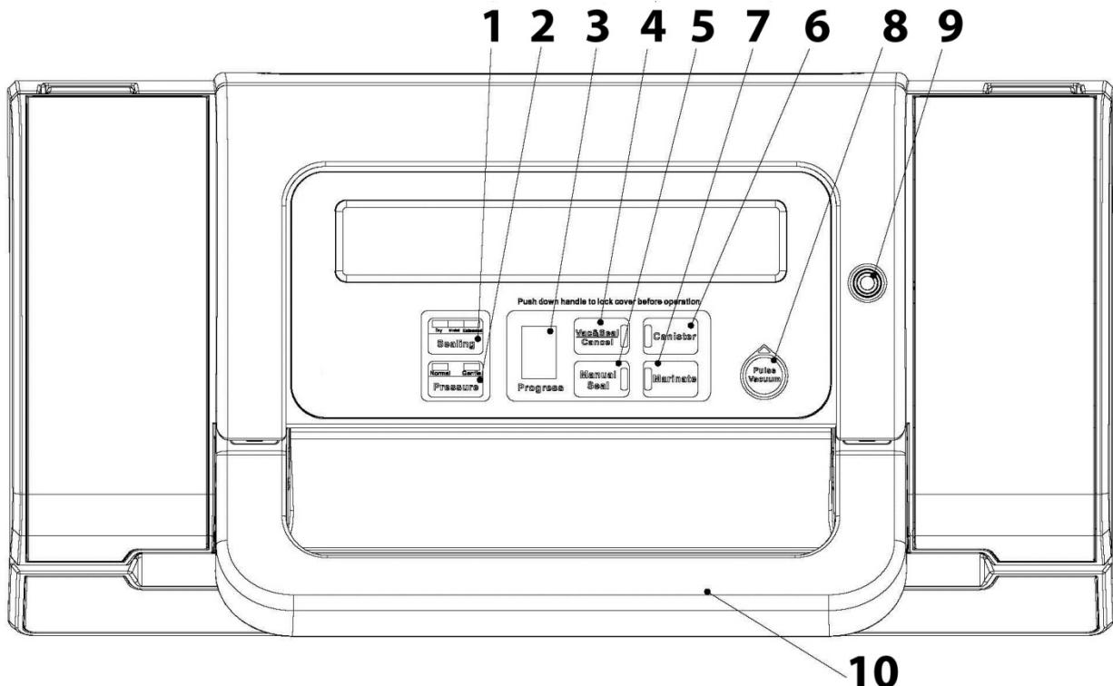
**9 Hose port:** To insert the hose for vacuuming canister or wine stopper.
